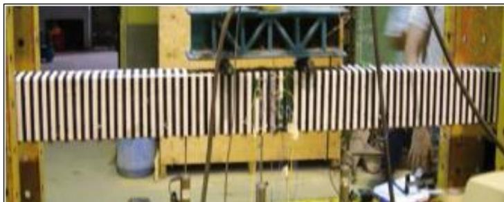
Figure 6. Final view of a typical HSC beam after strapping using the SSTT (Ma et al. 2016a)
