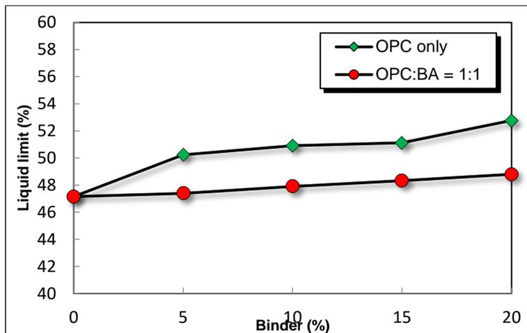
Figure 4. Variation of liquid limit of landfill soil with OPC and BA content
