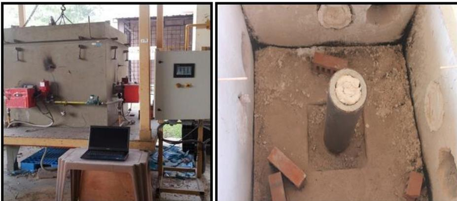
**Figure 10.** Fire furnace and CFDST column inside fire furnace
