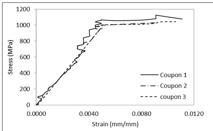
**Figure 3.** Measured stress-strain curves of steel straps (Ma et al., 2014a)
