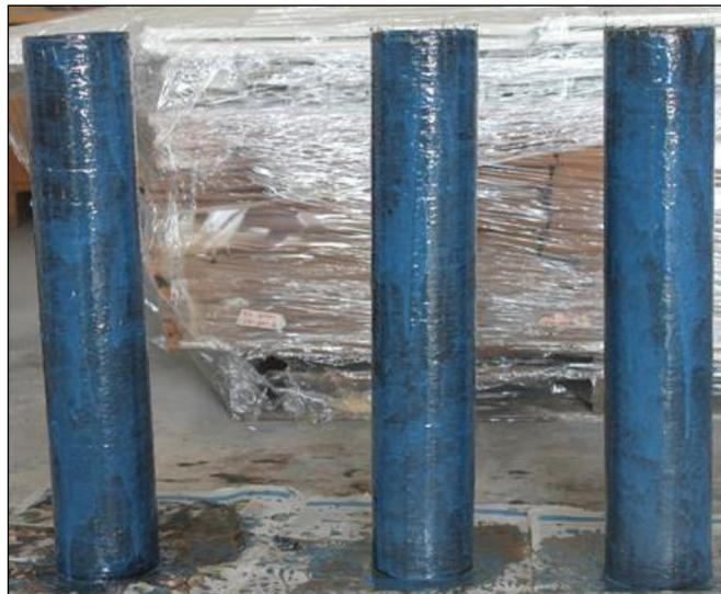
Figure 11. CFDST columns after repair
