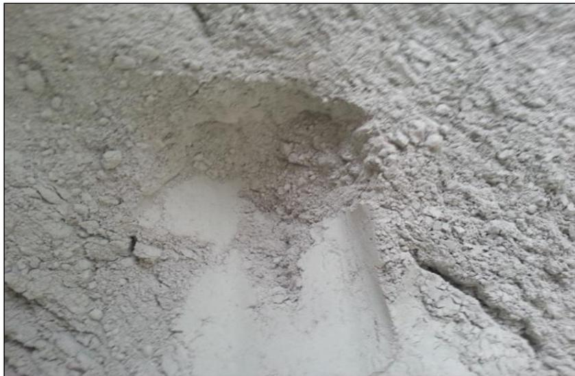
**Figure 3.** Quarry dust waste after grinding process
