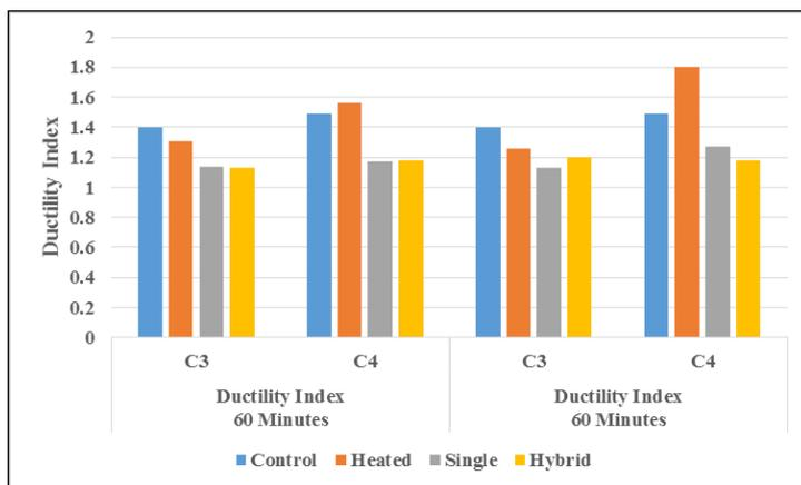
Figure 15. Ductility Index of repaired fire-damaged CFDST columns with Hybrid FRP
