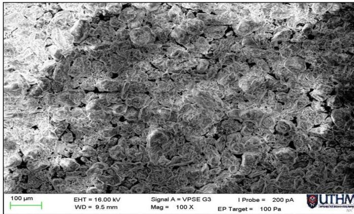
Figure 4. SEM micrograph for sand at 100x magnification
