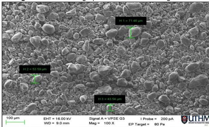
Figure 5. SEM micrograph for rubber ash at 100x magnification
