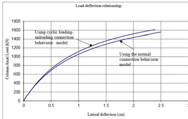
Figure 7. Load-deflection relationship at mid-height of the centre column
