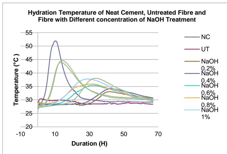
**Figure 5.** Hydration temperature of Neat Cement (NC), Cement-*EFB* Fibre (Untreated (UT), 0.2%, 0.4%, 0.6%, 0.8%, 1%, 2%, 3% and 4% of NaOH Treatment)
