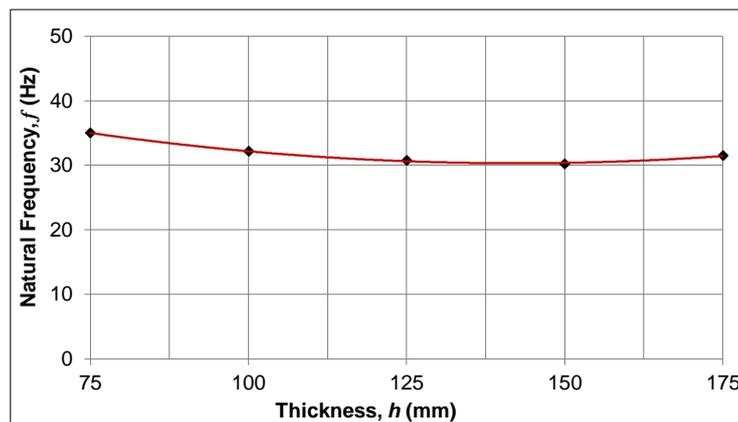
Figure 13. Natural frequency of composite slab at different thicknesses
