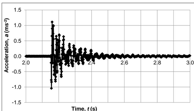
Figure 11. Acceleration-time history of composite slab CS-125
