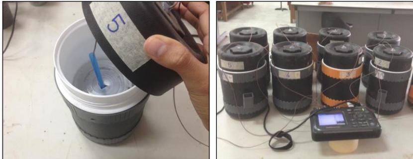
Figure 1. Hydration test setup and recorded
