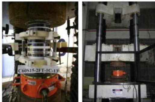
Figure 5. STT-confined specimens tested under cyclic loading (Lee et al. 2014)
