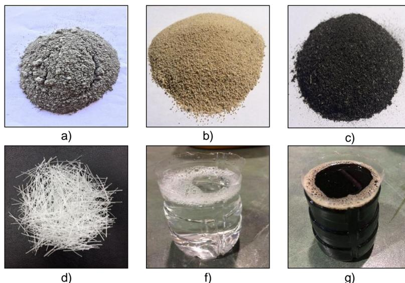
**Figure 2.** Main materials in foamed concrete; a) OPC, b) Sand, c) RHA, d) PMM), f) Foam agent and g) SP
