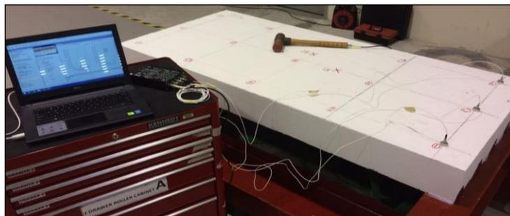
**Figure 7.** Test set-up for hammer-impact test
