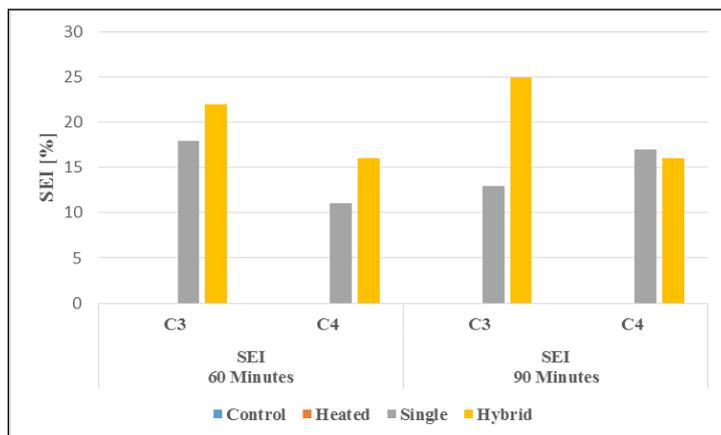
Figure 13. Strength Enhancement Index of repaired fire-damaged CFDST columns
