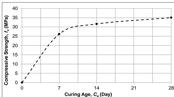
Figure 9. Compressive strength of foamed concrete containing 40% RHA and 9kg/m<sup>3</sup> PMM
