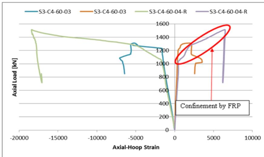
Figure 17. Confinement effect of single layer CFRP for 60 and 90 minutes of fire exposure time
