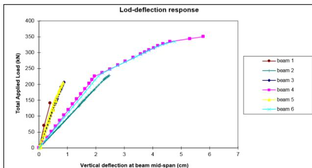
Figure 12. Load-Deflection relationship at the mid-span beam obtained from the developed analysis procedures
