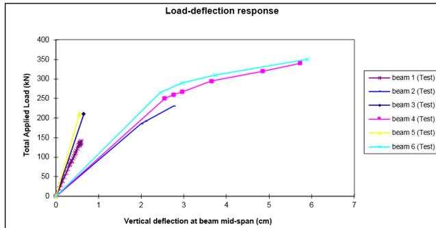
Figure 11. Load-Deflection relationship at the mid-span beam obtained from test results
