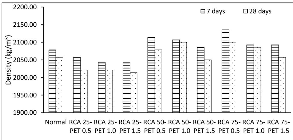
Figure 6. Density of Composite Bricks for 7 and 28 Days
