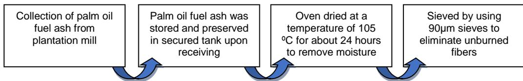
**Figure 2.** Palm oil fuel ash process before being used
