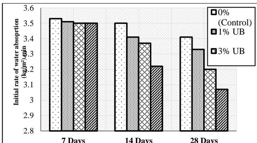
Figure 2. Initial water absorption of control and bacterial ICEB
