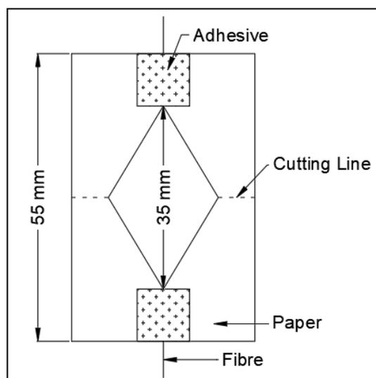
Figure 2. Schematic sketch of the experimental setup for tensile test
