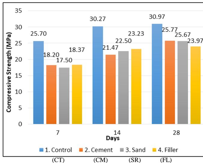
Figure 7. Compressive Strength of Cement Mortar against Time
