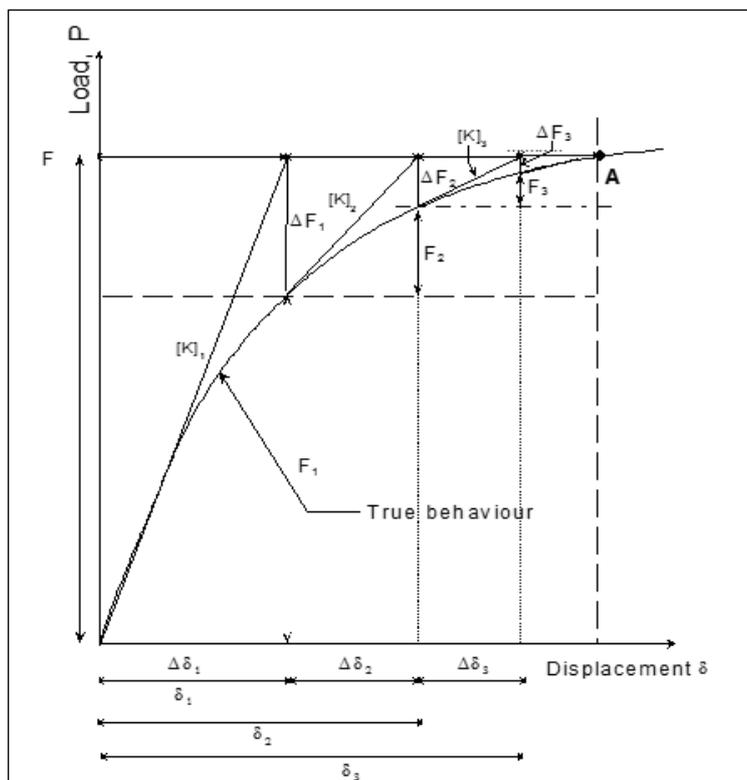
Figure 2. Newton-Raphson procedure of load-displacement relationships
