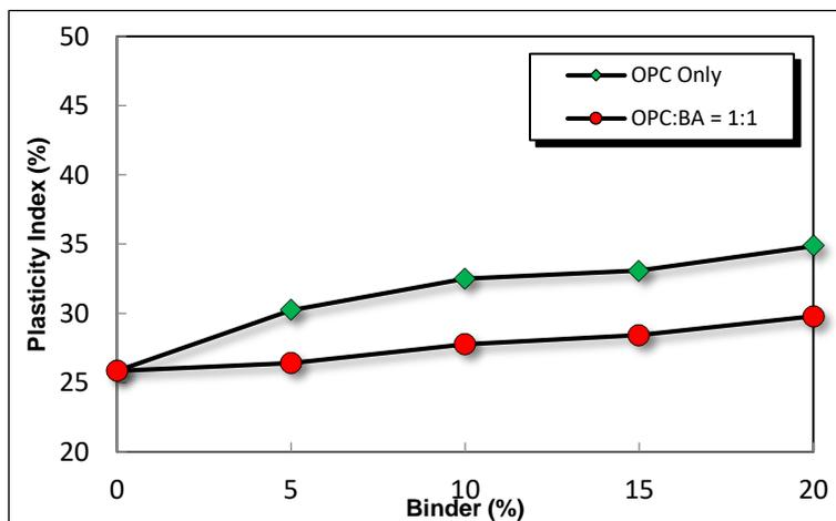
Figure 6. Variation of plasticity index of landfill soil with OPC and BA content
