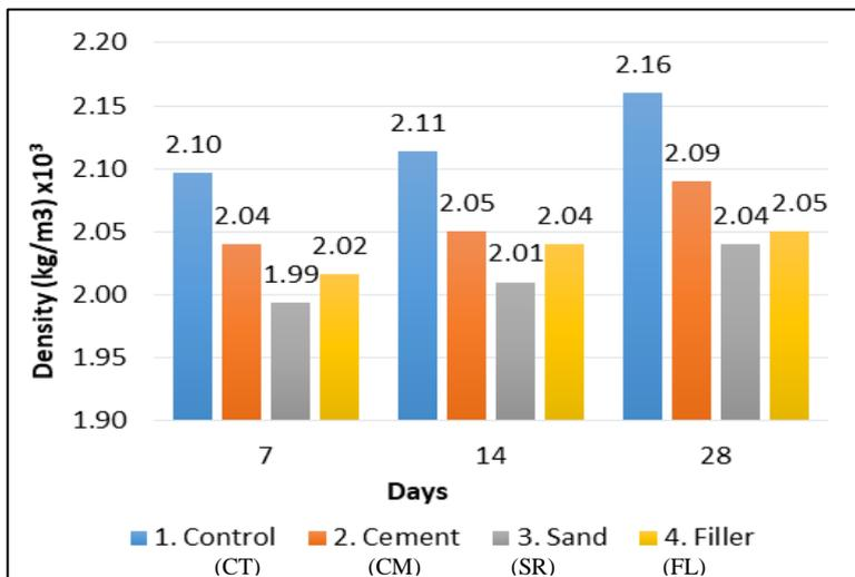
Figure 6. Graph Density of Cement Mortar Against Time
