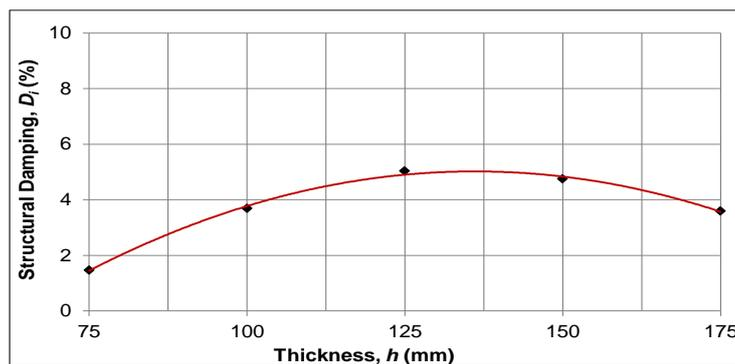
**Figure 14.** Structural damping of foamed concrete composite slab at different thicknesses
