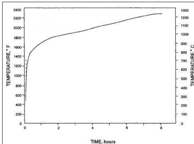
**Figure 9.** ASTM E-119 time-temperature curve
