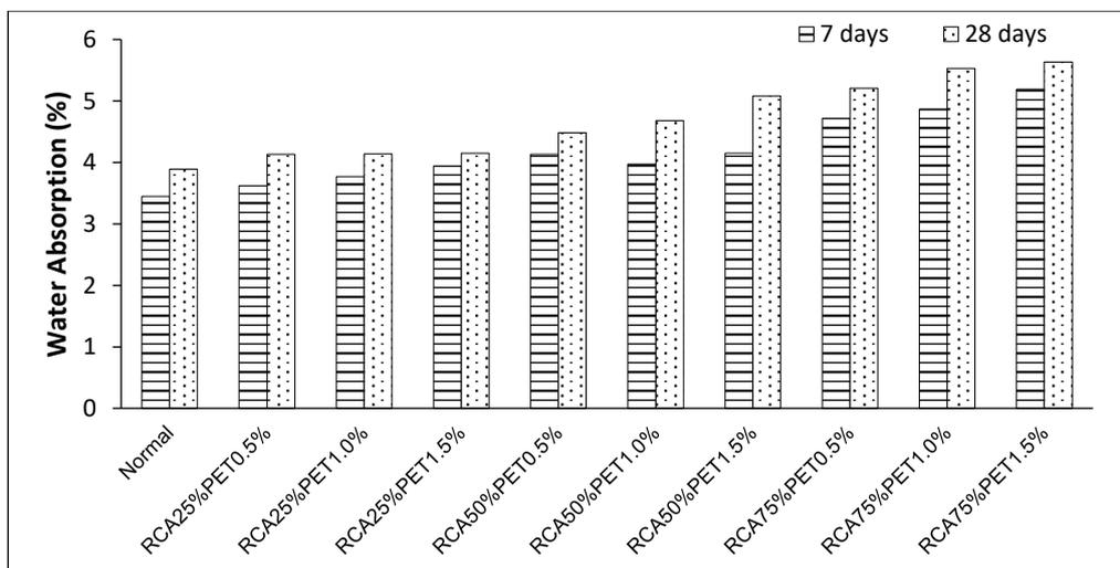
**Figure 10.** The average water absorption of sand cement composite bricks with RCA and PET
