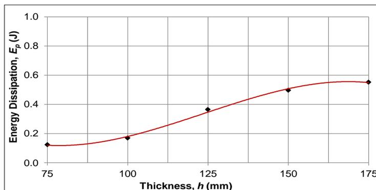
Figure 15. Energy dissipation of composite slab at difference thicknesses
