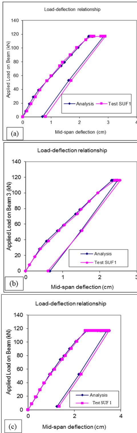
**Figure 17.** Comparison of the beam load-deflection response for SUF 1 at (a) Beam 2 (b) Beam 3 and (c) Beam 4
