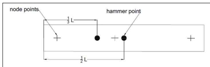
Figure 4. Hammer Point for Impact
