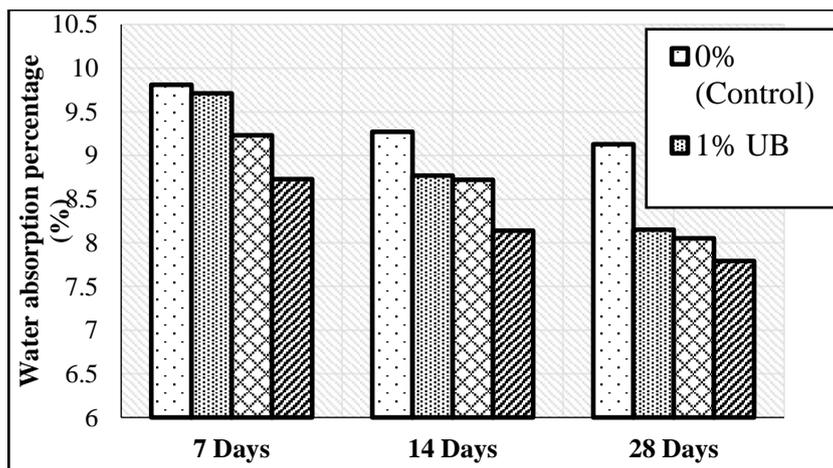
Figure 3. Percentage of water absorption by 24-hour soaking for control and bacterial ICEB
