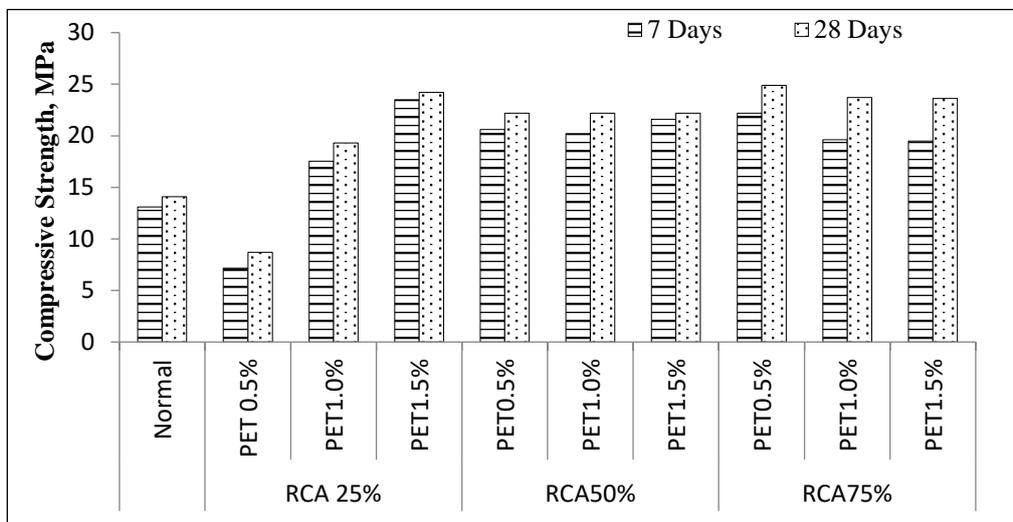
**Figure 8.** Compressive strength for 7 and 28 days
