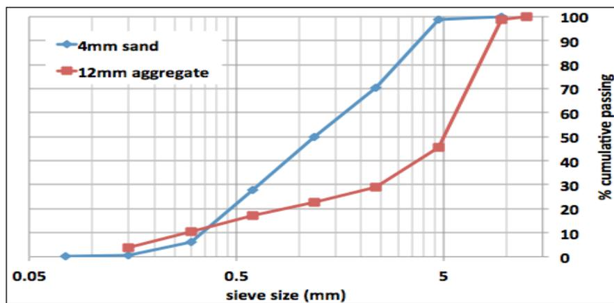
Figure 1. Sieve analysis for 4 mm natural river sand and 12 mm aggregate
