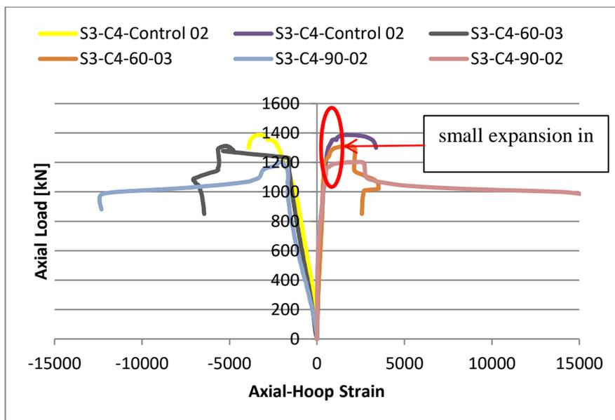
**Figure 16.** Axial load versus axial-hoop strain curves of Series 3 with  $t_0 = 4$  mm
