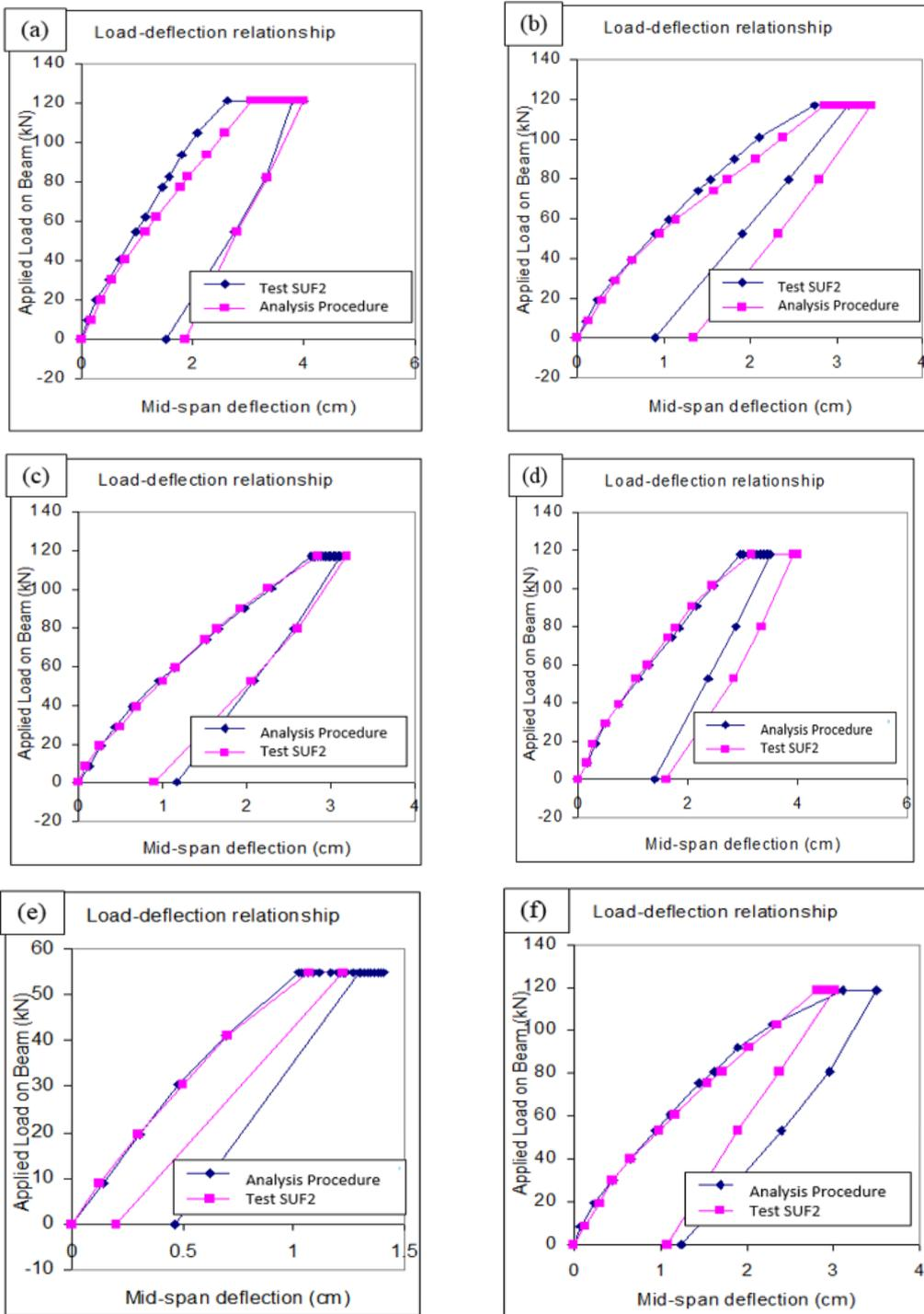
Figure 18. Comparison of the beam load-deflection response for SUF 2 of (a) Beam 1 (b) Beam 2 (c) Beam 3 (d) Beam 4 (e) Beam 5 (f) Beam 6
