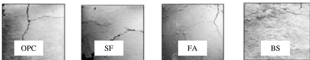
**Figure 3.** Surface cracking of concrete at 800°C (Poon et al.,2001)
