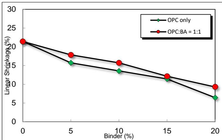
Figure 7. Variation of linear shrinkage of landfill soil with OPC and BA content
