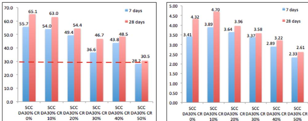
**Figure 7.** Compressive strength and tensile strength for SCC DA30% CR%
