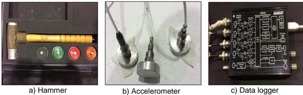
**Figure 6.** Instrument of hammer-impact test
