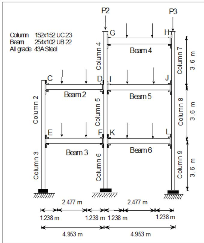
Figure 15. General arrangement of the frames SUF1
