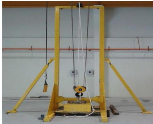
**Figure 3.** Drop weight Impact test equipment
