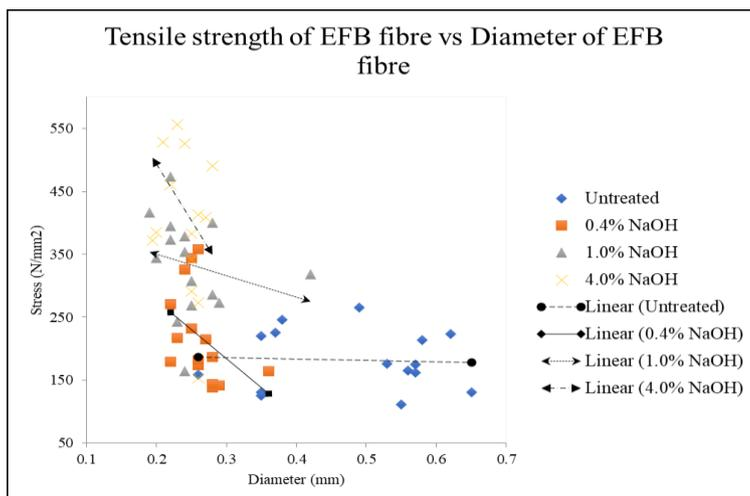
**Figure 8.** Tensile strength of EFB fibre againsts diameter for untreated and treated fibre
