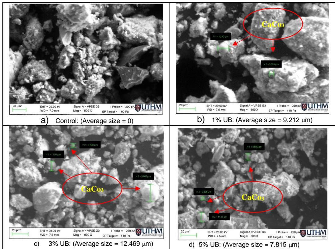
**Figure 5.** Precipitation of calcium carbonate for control and bacterial ICEB
