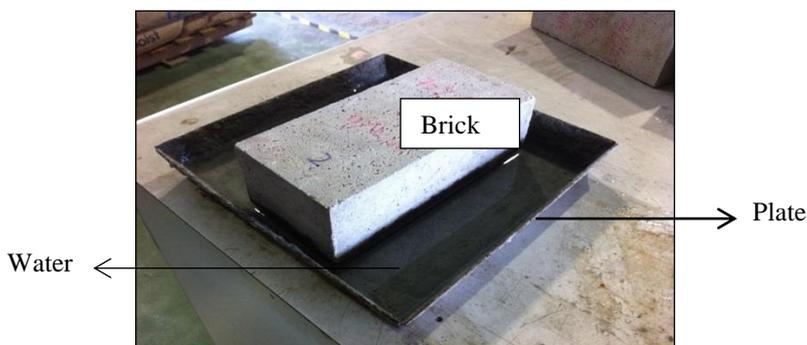
**Figure 5.** Initial rate of suction test
