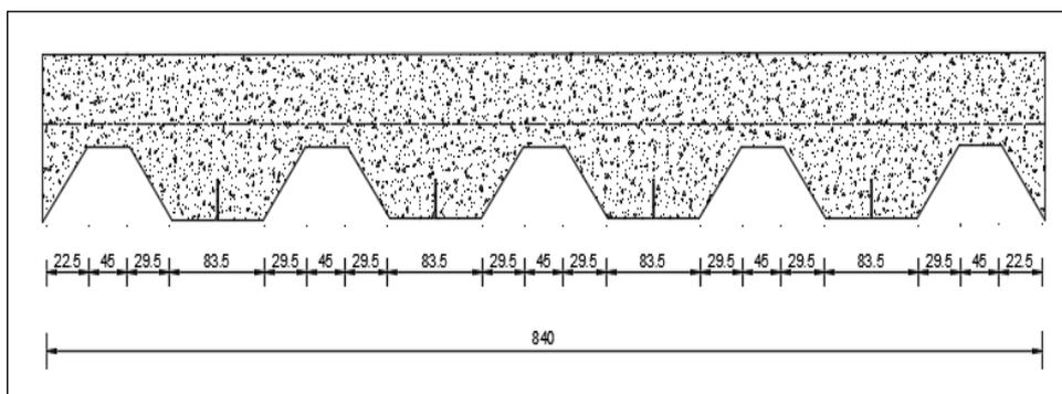
**Figure 3.** Schematic design of composite slab
