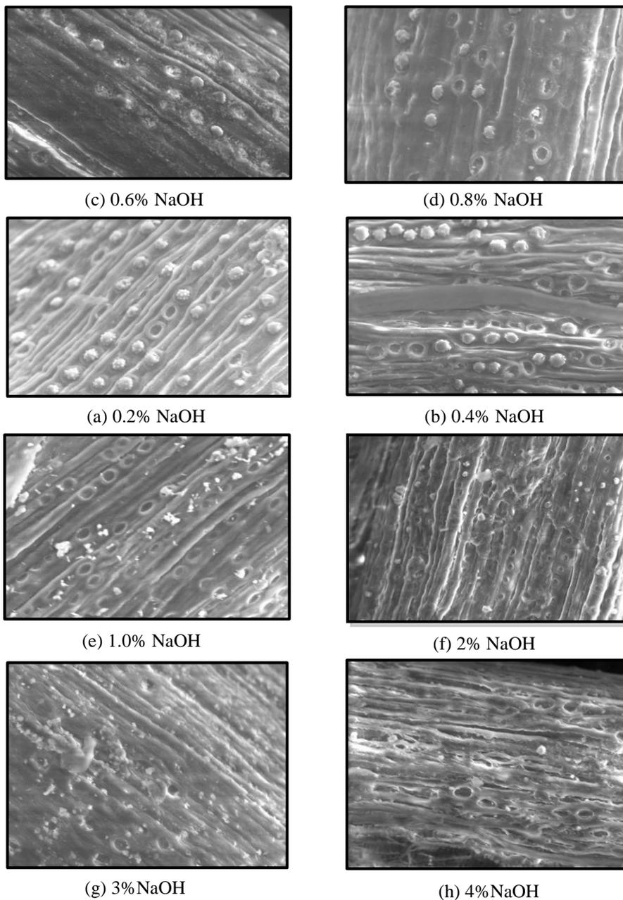
**Figure 4.** Scanning Electron Microscope (SEM) image at 250 magnification of Oil Palm Empty Fruit Bunch (OPEFB) treated with Sodium Hydroxide (NaOH) range 0.2% to 4% concentration
