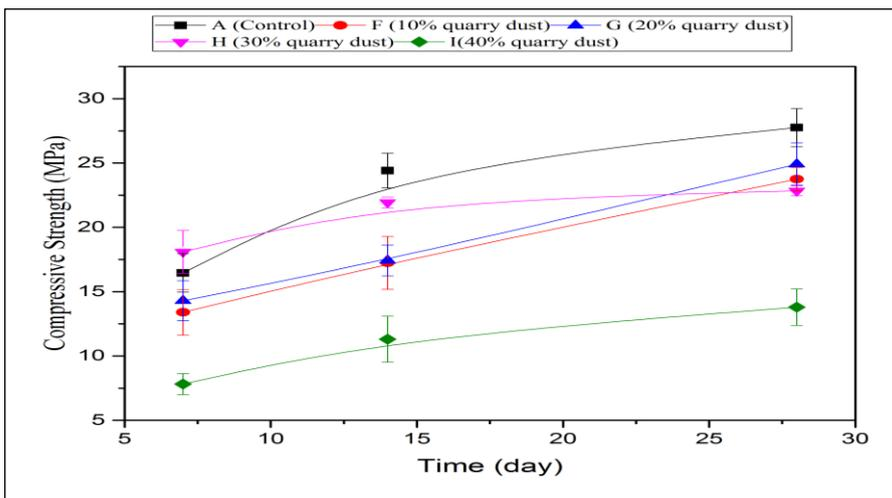
Figure 8. Compressive strength of various percentages of quarry dust with 0% (control), 10%, 20%, 30% and 40% at different ages (7, 14 and 28 days)
