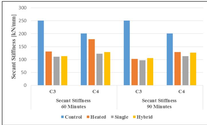
Figure 14. Secant stiffness of repaired fire-damaged CFDST tubular columns with Hybrid FRP
