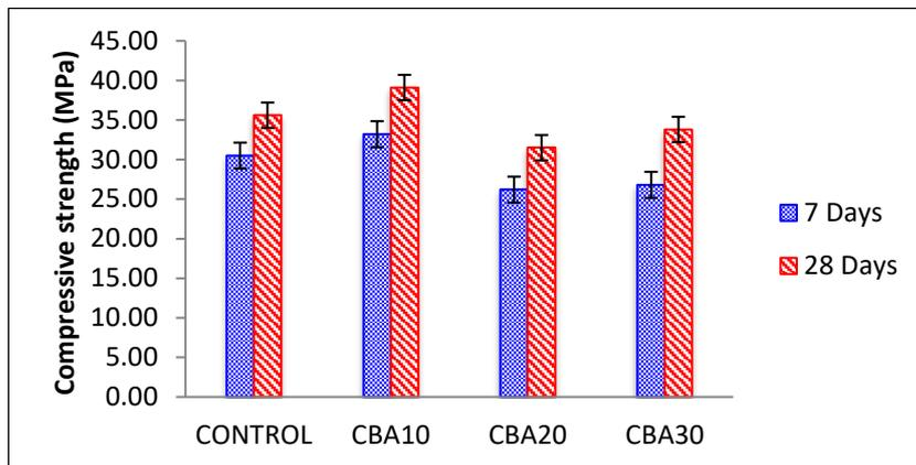
**Figure 6.** Compressive strength of concrete containing various CBA percentage for 40 hours grinding time
