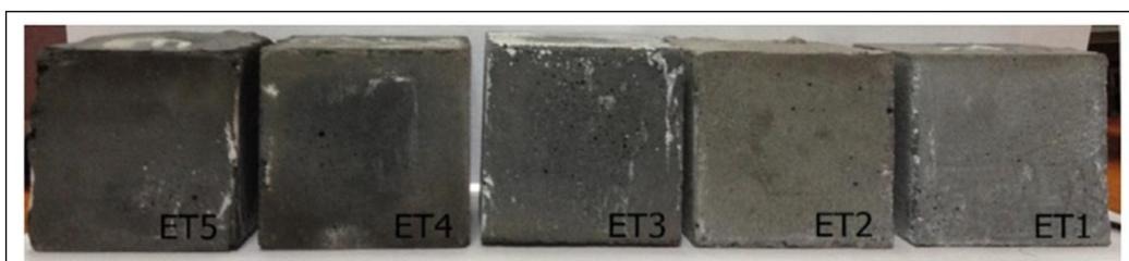
Figure 4. Effect of temperature on discolouration of concrete (Ranjbar et al., 2014)
