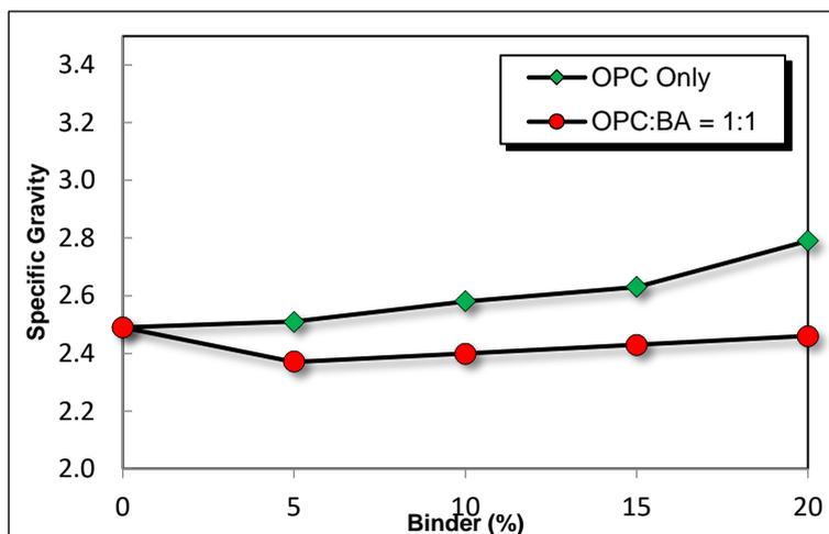
Figure 3. Variation of specific gravity of landfill soil with OPC and BA content
