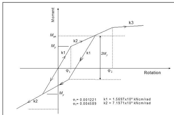
Figure 6. Moment-rotation characteristic for connection used in the frame shown in Figure 6
