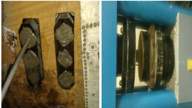
**Figure 3.** Preparation of mortar cubes and the compression test equipment
