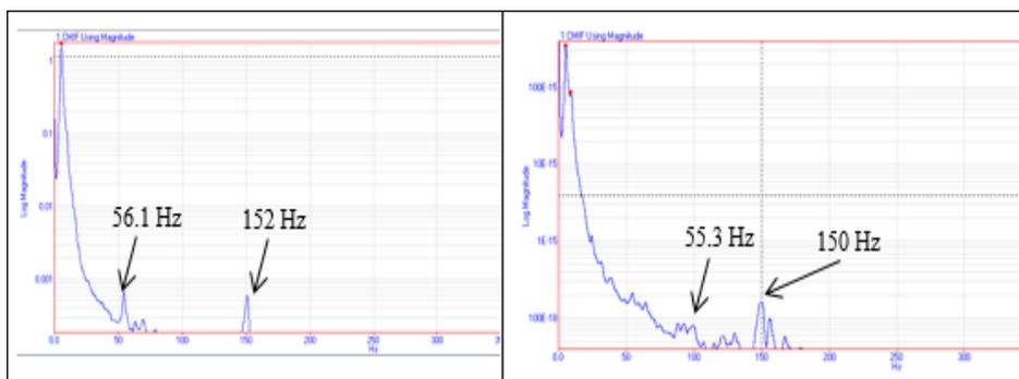
**Figure 6.** Natural frequency of beam before and after strike of 15 kA of electric current
