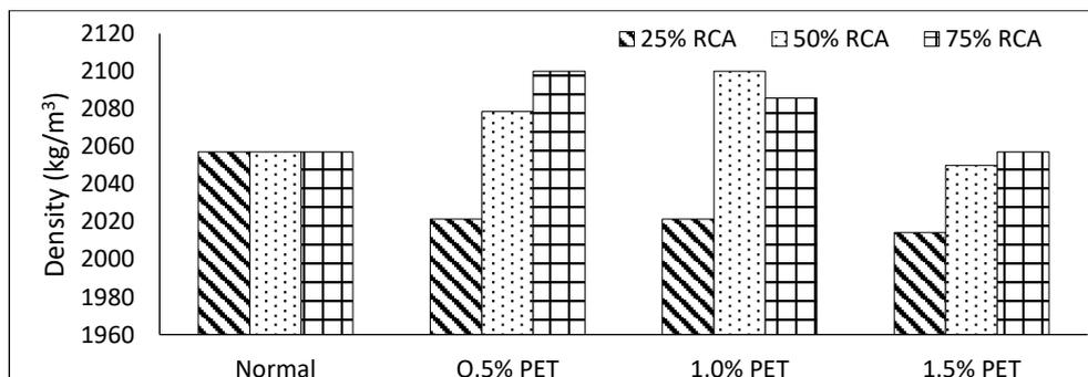
Figure 7. Density of Composite Bricks according to RCA content at 28 Days
